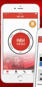
The 'Help Me' button sends an emergency text with GPS location details to two nominated mobile numbers
